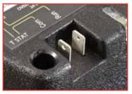
Two wires with pre-crimped connectors may be plugged onto the COMMON and RUN terminals and wired into the 24 Volt thermostat circuit to shut off A/C systems should an overflow condition occur. The Safety Switch operates with or without power provided to the pump.
