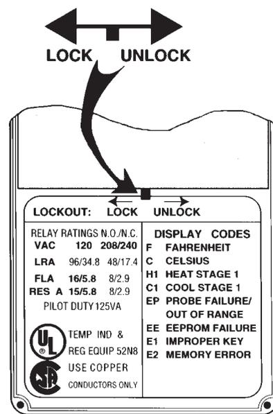
**Figure 2: Lockout Switch**
