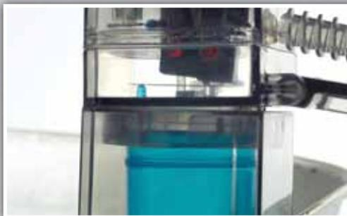
**Reliable Mechanical Contact Float Switch**
