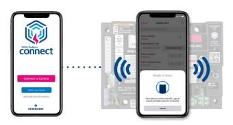
**Near Field Communication (NFC)** creates an interface between the control and your mobile device with the White-Rodgers Connect app. Place mobile device in contact with the NFC marking on module to enable a connection.
