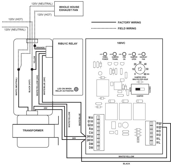
The iO-FAVR-ENHANCED has a built-in transformer used to power the outside air damper open when the panel calls for ventilation air and a relay that allows a whole house exhaust fan to be wired directly to the panel. Whenever the FAVR calls for ventilation air, 24 volts is sent to the relay coil which closes the 120V (Hot) contact to the exhaust fan.
