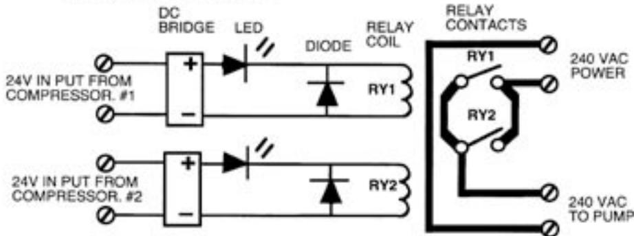
EITHER COMPRESSOR #1 OR COMPRESSOR #2 WILL START PUMP
