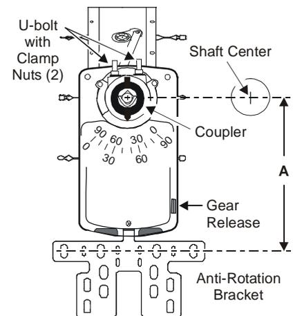
**Note:** A is the distance from the center of the holes in the anti-rotation bracket to the center of the shaft. (See Table 1.)
