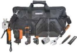
**NAVAC Advanced Tool Kit for Mini-Split Installation**
