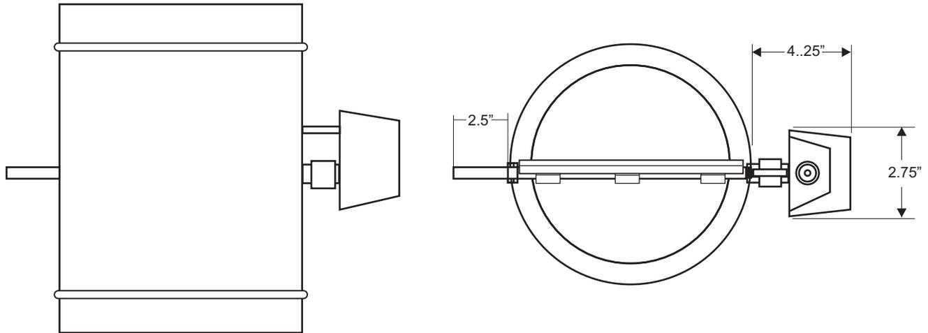
The OAD-XX is designed for retrofit or new construction applications requiring exhaust, fresh air intake and on-off zone control. Typical application use includes bathrooms or restrooms in high rise hotels, office buildings and apartment buildings. The damper is available with a direct coupled, spring return actuator in 24 VAC or 120 VAC, and an accessory plate is available for actuator mounting.
