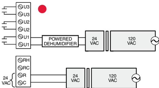
Typical hookup of variable speed blower for dehumidification in low speed
