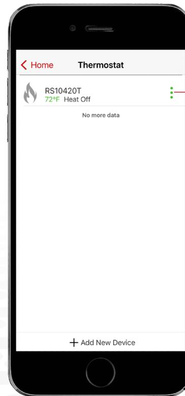
The active **RS10420T** displays the current temperature in green. Tapping the active thermostat reveals settings seen in **Step 4**.
