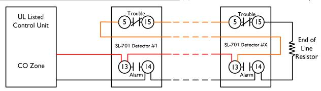
SAMPLE ADDRESSABLE PANEL WIRING - STYLE "6"/CLASS "B" SLC (Supervised - A fault condition will not inhibit an alarm response)
