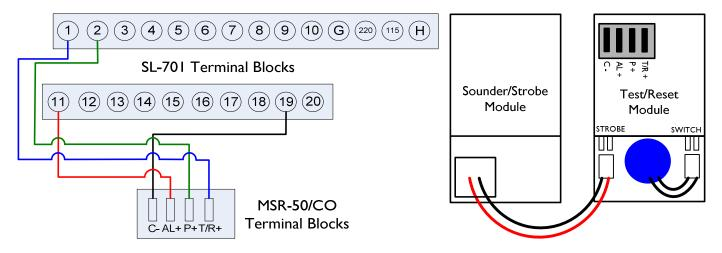
The SL-701 provides a 2 amp form "A" alarm contact and a 10 amp form "C" trouble contact for fire alarm control unit monitoring. The SL-701 will give a trouble report if the unit loses power, if the cover is removed, a sensor "end of life", or improper installation of the sensor.
