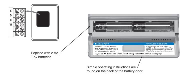
**NOTE:** In applications where the thermostat will see temperatures below 40 degrees it is recommended that 1.5V AA lithium batteries be used instead of alkaline for increased battery life. (Extreme temperatures decrease the life of Alkaline batteries.)
