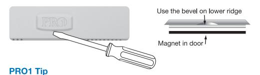
Gently slide a screwdriver into the bottom edge of the badge. Gently turn the screwdriver counter clockwise. The badge is held on by a magnet in the well of the battery door. The badge should pry off easily. Do not use force.
