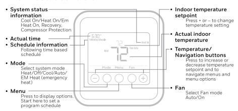
The screen will wake up by pressing any of the five buttons. If powered by the C wire, the screen stays lit for 45 seconds after you complete changes. If powered by battery only, the screen stays lit for 8 seconds. Depending on how your thermostat was installed, the screen light may always be on.
