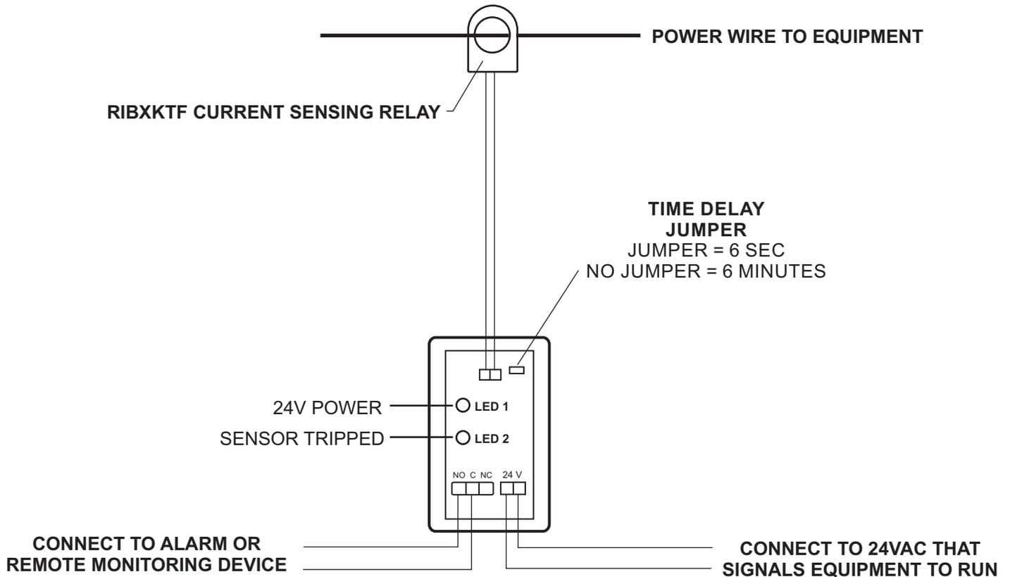
The UMM-CS can monitor the current to a HVAC blower using a current sensing relay. If no current is detected after 6 seconds, the relay contacts can be used to trigger an alarm or remote monitoring device. Make sure to connect 24VAC to the UMM that signals equipment to run.
