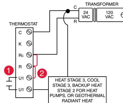
● U1 terminals are normally open dry contacts when set up for a stage of heating or cooling.
