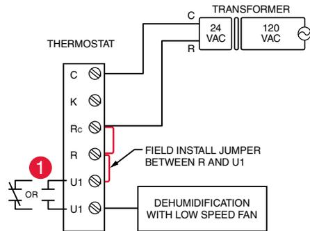
● Wire the thermostat universal relay to the low speed fan for dehumidification control at the equipment. The thermostat relay can be set to normally open or normally closed in the thermostat installer setup.
