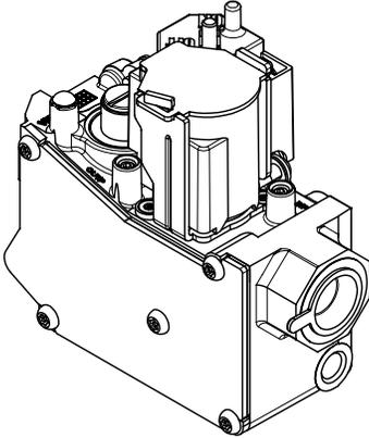
This control has a standard opening characteristic, which is suitable for a wide range of applications. It provides a fast rise to full pressure upon energizing the solenoid. Regulator LP spring conversion kits are available for this control.
