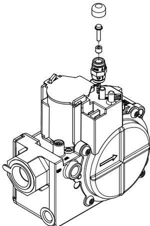
The convertible regulator option for this control involves a construction, which permits easy Natural to LP conversion (or vice versa) by removing, inverting and replacing the regulator cap screw. This feature easily lends itself to use in mobile homes and infra-red applications
