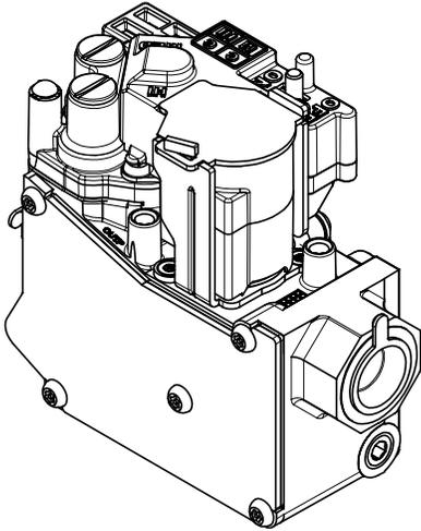
This control has dual outlet pressure levels, which is desirable for high efficiency applications. It provides a fast rise to first stage pressure upon energizing the single stage solenoid. Then, if more pressure level is required to satisfy heating requirement, energizing a second stage solenoid can attain a higher pressure level. Regulator LP spring conversion kits are available for both pressure levels on this control.
