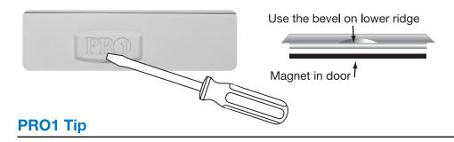
Gently slide a screwdriver into the bottom edge of the badge. Gently turn the screwdriver counter clockwise. The badge is held on by a magnet in the well of the battery door. The badge should pry off easily. **Do not use force.**
