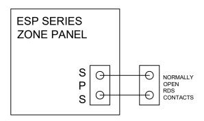
**NOTE:** All zones must be set to ESP ON via jumper or LCD display
