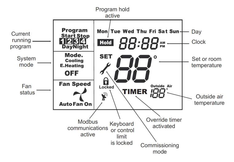
The T-32-P is capable of many advanced control options. Not all LCD symbols may appear on your specific thermostat configuration.
