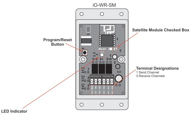
Communicating – Solid Green w/ Blinking Red Every 15 Seconds Loss of Communications – Solid Red
