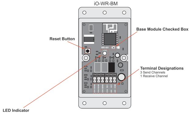
Communicating – Solid Green w/ Blinking Red Every 15 Seconds Loss of Communications – Solid Red Ready to Pair with SM – Alternating Blinking between Green and Red
