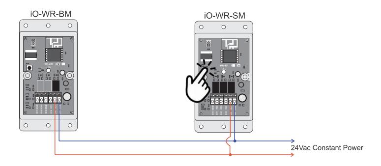
3. Remove power from the iO-WR modules and install each module in its intended location as far from metallic surfaces as possible.
