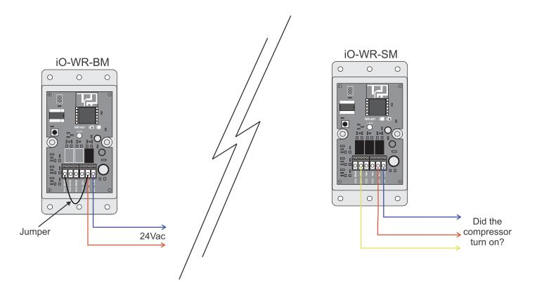
If the outdoor unit turned on, then there is likely a wiring issue at the indoor unit or an issue with the thermostat.
