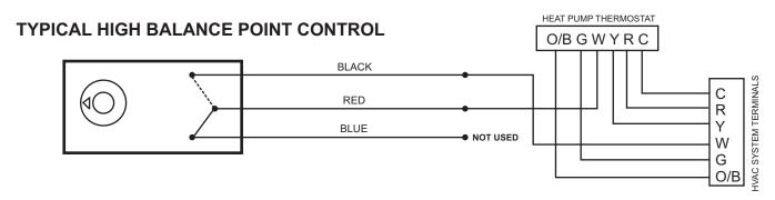
Used to prevent auxiliary heat from running when outdoor temperature is above a selected setpoint. Red and Black open above setpoint.
