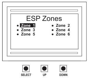
The factory default for all zones is active ESP function as indicated by the bullet (•) next to each zone. To deselect a zone, press the UP or DOWN button until the bullet disappears.
